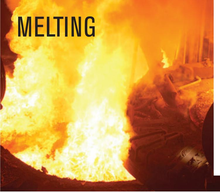
The Electric Arc Furnace allows to melt a metal charge with a high percentage of iron, in order to get liquid steel. The electric arc energy is transformed into heat and irradiated to the charge.
